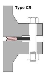
Solid metal outer ring used as a centerring device and compression stop.
