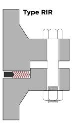
Solid metal inner ring. Use with high pressures and temperatures.
