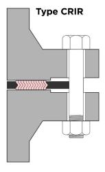
Solid metal outer and inner rings. For use at high pressures and temperatures.
